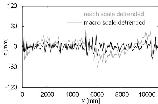
Figure 10. Illustration of data processing: After removal of reach-scale trend profile significant local trends caused by macro-scale bed features are still visible
