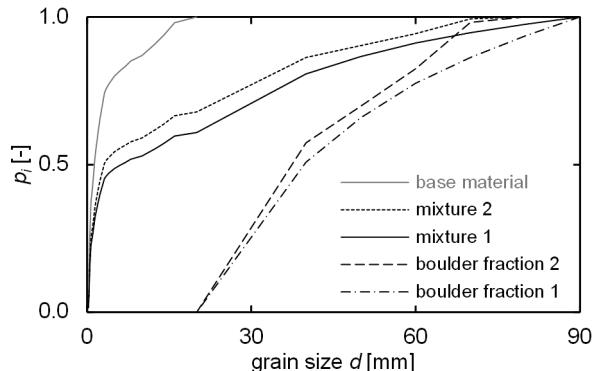
Figure 2. Grain size distribution of mixtures used
