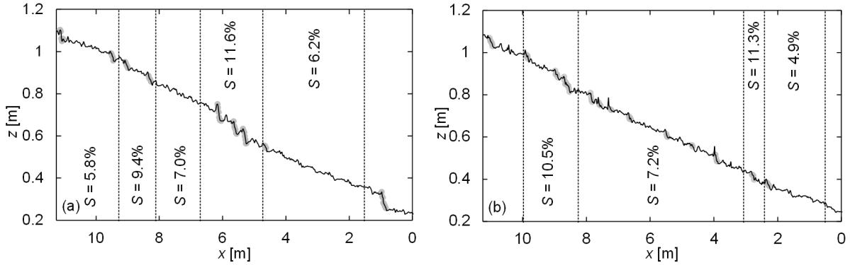
Figure 8. Mean longitudinal profile after  $HQ_{100}$  for test series (a) A1 and (b) A2. Step structures in meso-scale in grey. Dashed lines confine sequences of steep ( $>0.08$ ) and flat ( $<0.08$ ) slopes i.e. riffle-pool structures in macro scale. Reach-averaged slopes are 0.08 ( $\pm 0.002$ )
