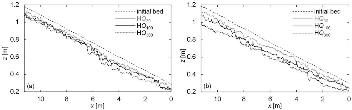
Figure 5. Evolution of longitudinal profile with increasing discharge for test series (a) A1 and (b) A2 with initial bed slope of  $S = 0.08$
