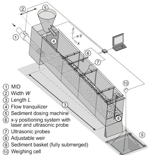
Figure 1. Schematic representation of model flume
