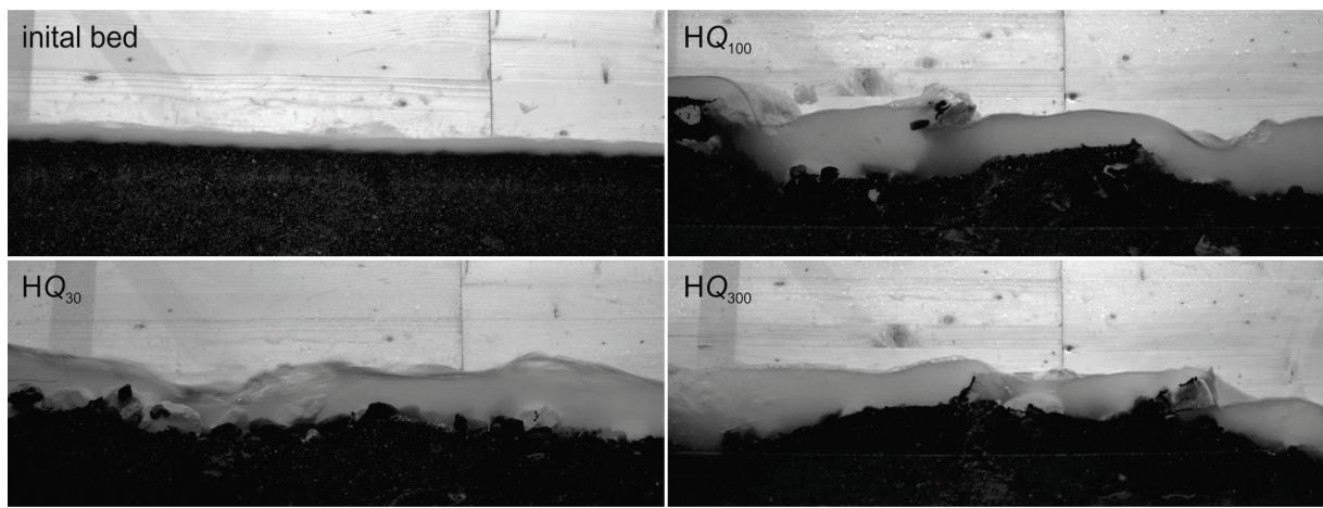
Figure 4. Side view of initial bed, during  $HQ_{30}$  event, after  $HQ_{100}$  and  $HQ_{300}$  peak flows. Flow direction from left to right
