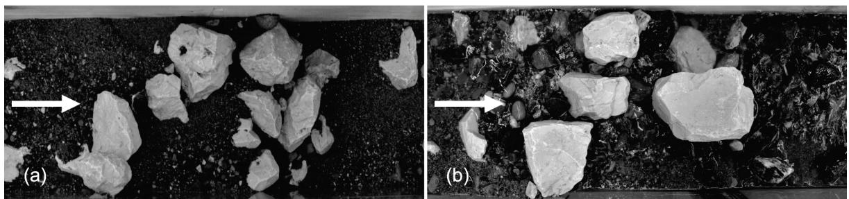
Figure 7. Picture of (a) tightly-interlocked step and (b) loose accumulation of large grains for test series A2 after HQ<sub>100</sub>.
