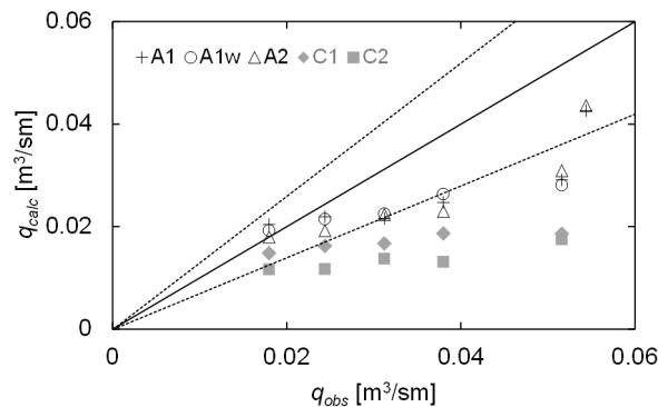
Figure 12. Comparison of measured bed forming discharges and values calculated with Eq. (2). Dotted lines represent  $\pm 30\%$  lines
