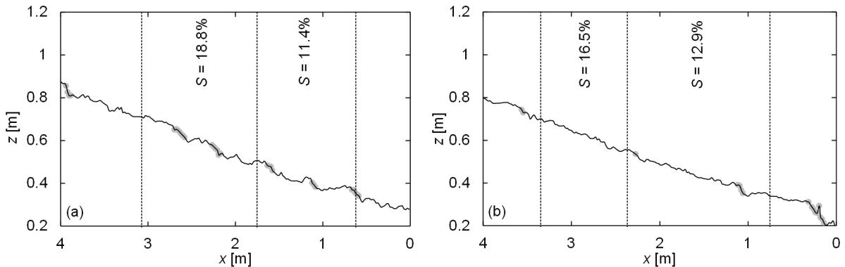
Figure 9. Mean longitudinal profile after  $HQ_{30}$  for test series (a) C1 and (b) C2. Step structures in meso-scale in grey. Dashed lines confine sequences of steep ( $>0.15$ ) and flat ( $<0.15$ ) slopes i.e. riffle-pool structures in macro scale. Reach-averaged slopes are 0.15 ( $\pm 0.002$ )
