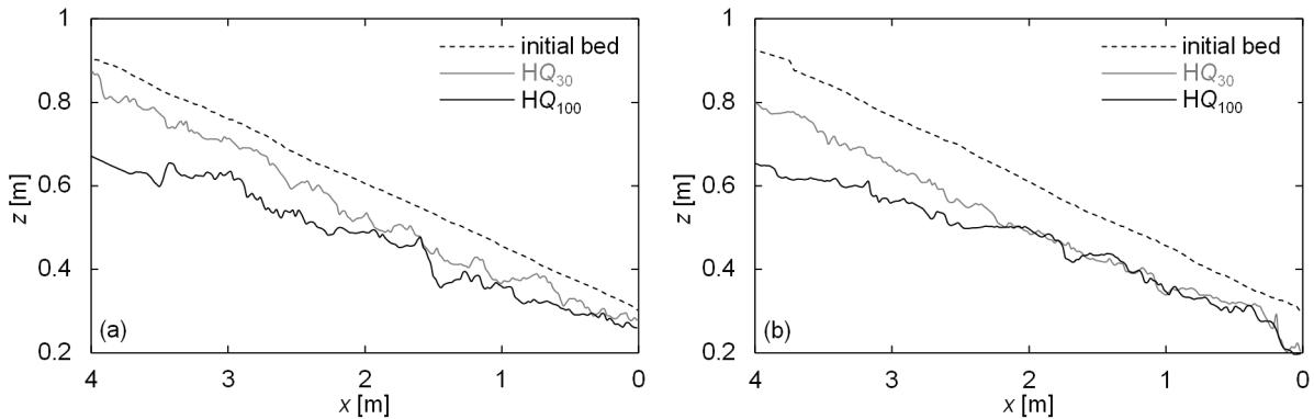
Figure 6. Evolution of longitudinal profile with increasing discharge for test series (a) C1 and (b) C2 with initial bed slope of  $S = 0.15$
