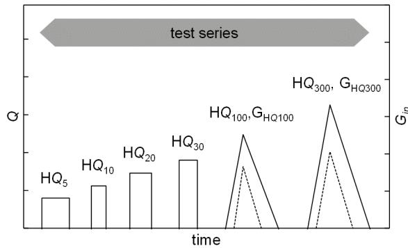
Figure 3. Illustration of experimental procedure. One test series consists out of six separate runs. Between each run the channel bed was scanned with laser probe. Note  $Q$  = water discharge and  $G_{in}$  = sediment input rate
