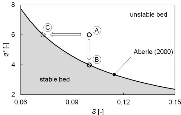
Figure 11. Illustration of different reach-scale stabilization mechanisms (adapted from Weichert 2006)
